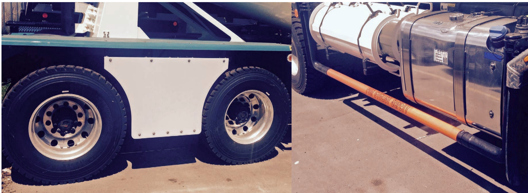
Innocon designed the Guardian, a safety device to protect cyclists and pedestrians from injury, and installed it on their Mack Granite.
