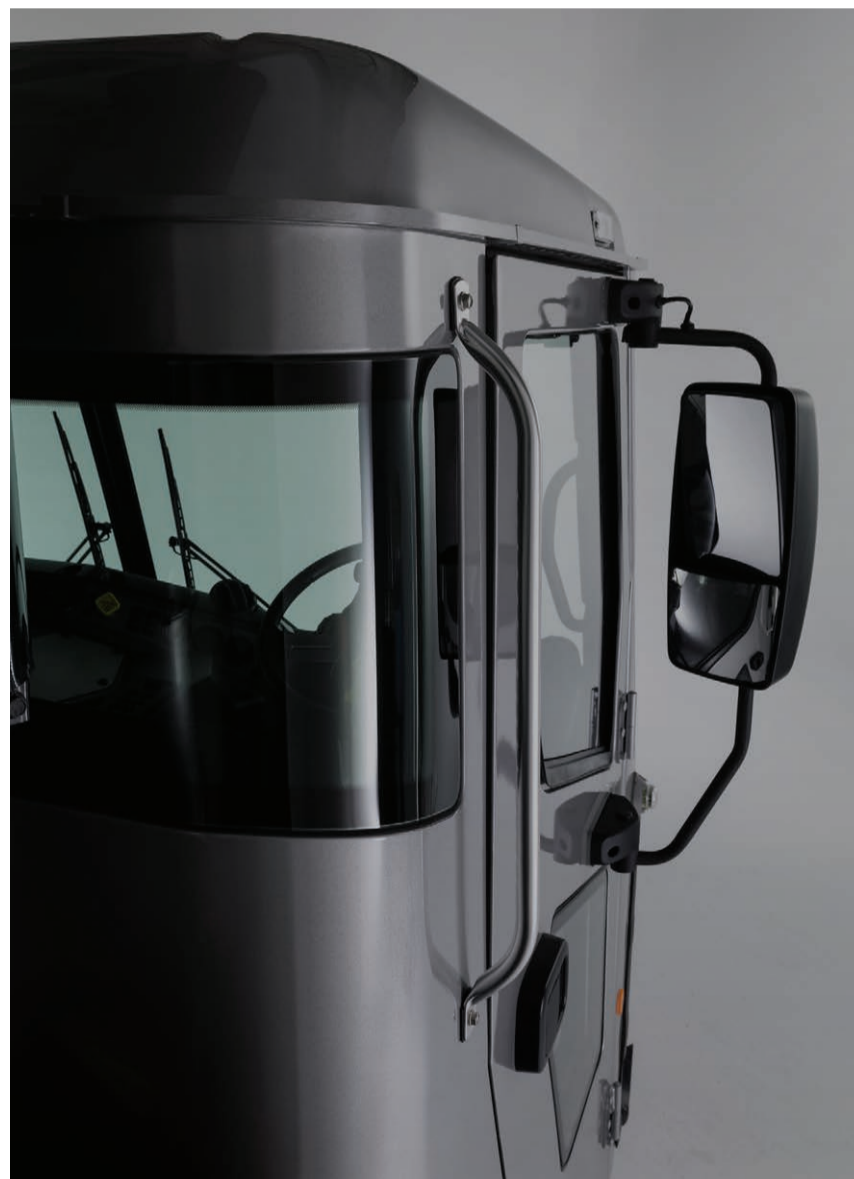
The LR series was designed with enhanced safety features, including larger glass in the cab to improve visibility and rear wraparound windows that increase the driver's field of vision.
