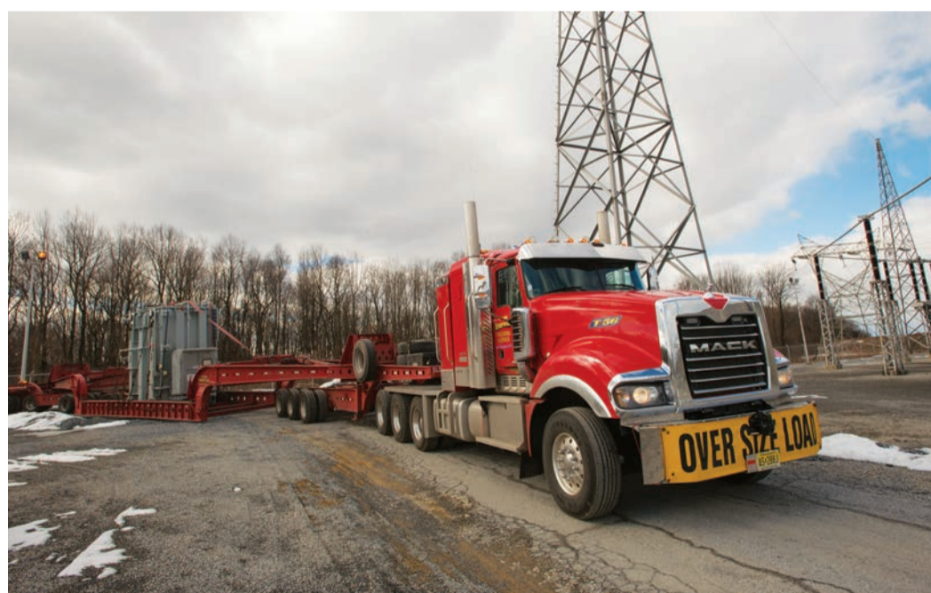
In early February, Trans American Trucking Services, South Plainfield, NJ, used a Titan by Mack to move several huge electrical transformers, also known as shunt reactors, from a terminal in Philadelphia to a Pennsylvania Power & Light substation in Lower Macungie, Pennsylvania (coincidentally, just down the road from Mack Trucks Lehigh Valley Assembly Operations). Each transformer weighed 133,600 pounds and required a 13-axle perimeter frame lowboy. The Titan was unfazed by the conditions created by a big snowstorm followed by rain a few days earlier, and handled the muddy destination with aplomb.
